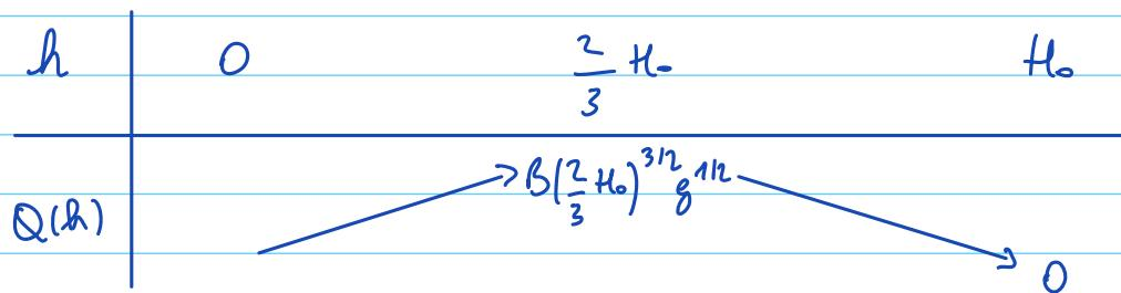
$$\begin{aligned} \text{en effet } Q\left(\frac{2}{3}H_0\right) &= B \frac{2}{3}H_0 \sqrt{2(H_0 - \frac{2}{3}H_0)g} \\ &= B \left(\frac{2}{3}\right)^{3/2} H_0^{3/2} g^{1/2} \end{aligned}$$
